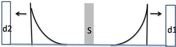
FIG. 2: Irby experiment. A positron is created in the source, S, and the time difference between annihilation photons arriving at detectors d1 and d2 is measured.
